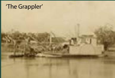
'The Grappler' was the earliest vessel to remove snags from the SA River Murray. Snags were chained up by a diving team and winched out of the river by a slewing crane. Explosives were used to dislodge stubborn snags.
