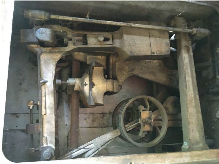
Weighbridge internal workings
