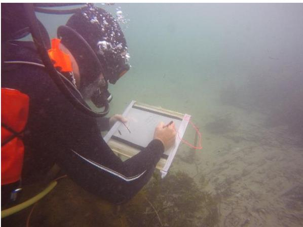
The team conducted a survey over a period of five days to locate the shipwreck site, and included reef walks with metal detectors to map the debris field and boat-towed magnetometer surveys.
