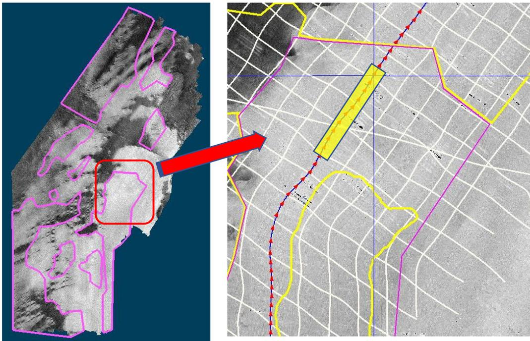
An offshore example from the SW corner of the 2020 survey area is shown below. In this case the polygon captures an area of seabed that shows variation in the backscatter intensity.
