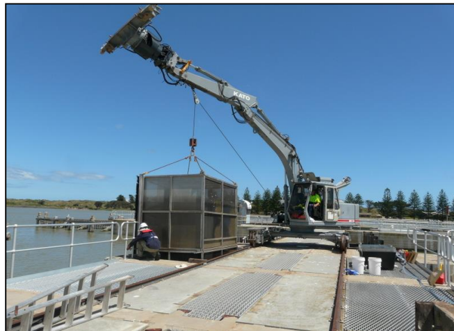
Figure 1. a) Trap used to sample the Tauwitchere Barrage small vertical-slot fishway and b) the large vertical-slot fishway trap being deployed at Goolwa Barrage.
