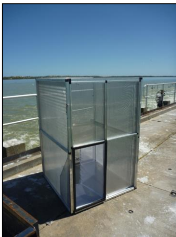
Figure 1. a) Trap used to sample the Tauwitchere Barrage small vertical-slot fishway and b) the large vertical-slot fishway trap being deployed at Goolwa Barrage.
