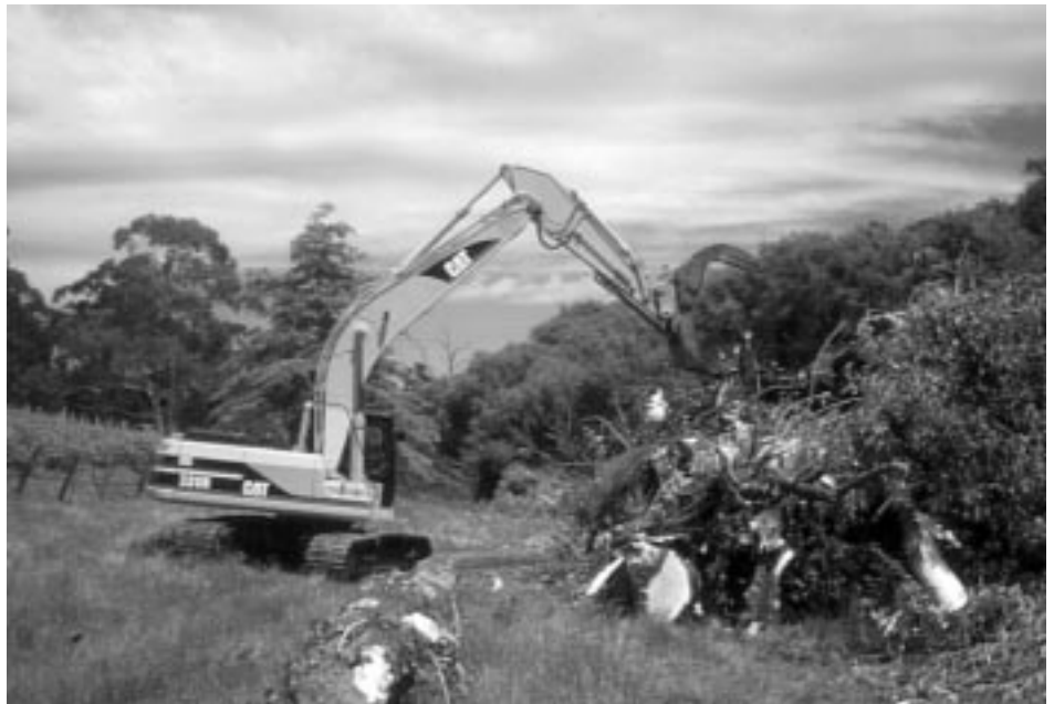
Where funds are available, the use of an excavator with a log grab to stockpile the fallen trees has proved to be cost effective and efficient method of willow removal
