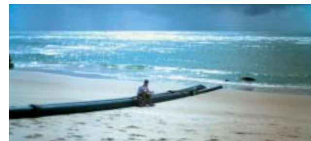
Example of sand acquisition pipeline (Noosa, Queensland)
